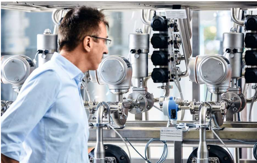
Uwe Rutsch, Head of Development and Product Management from SED Flow Control, in front of the test bench for diaphragm valves.
