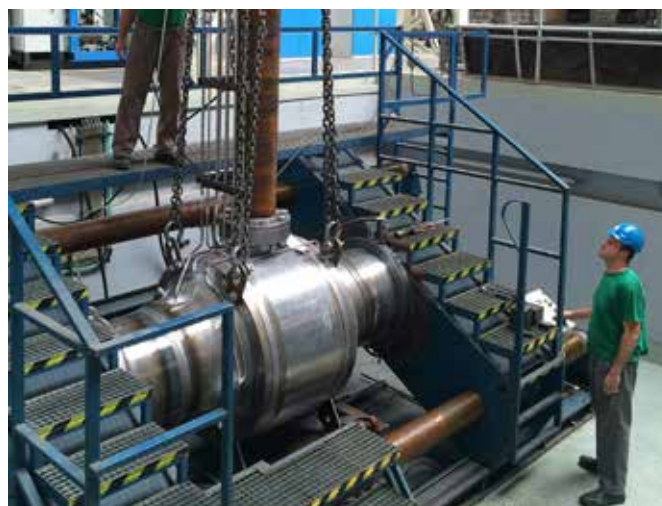
Pressure test of ball valves at our workshop
