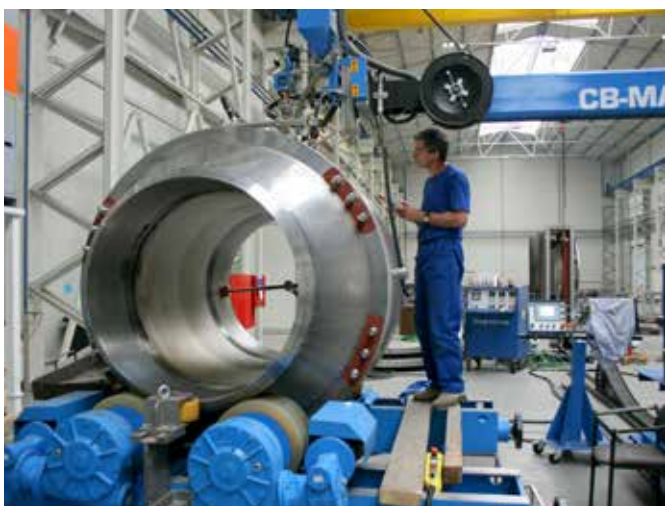
Automatic welding of ball valves DN 1400
