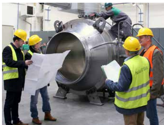
Inspection of ball valves DN 1400 for Eustream, Slovakia
